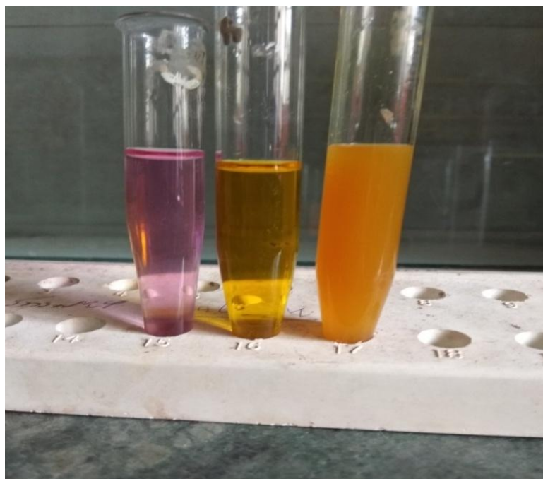
Fig. 1. Colour dispersion before and after nanoparticles formation (i) Final gold dispersion formed after reduction HAuCl 4 solution (ii) HAuCl 4 solution (iii) HAuCl 4 solution with extract before reduction
